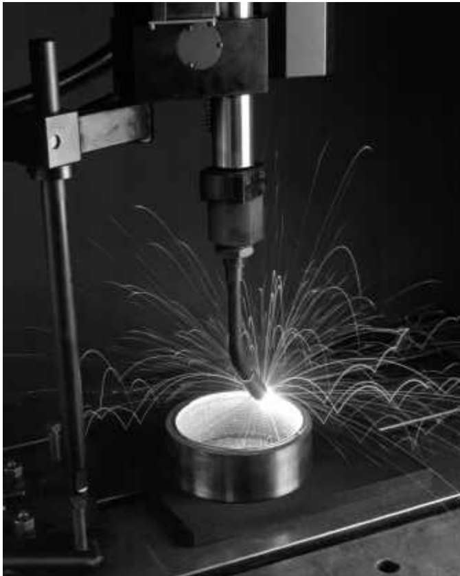
The Bortech BoreWelder in operation is ideal for repairing worn diameters without bushings.
